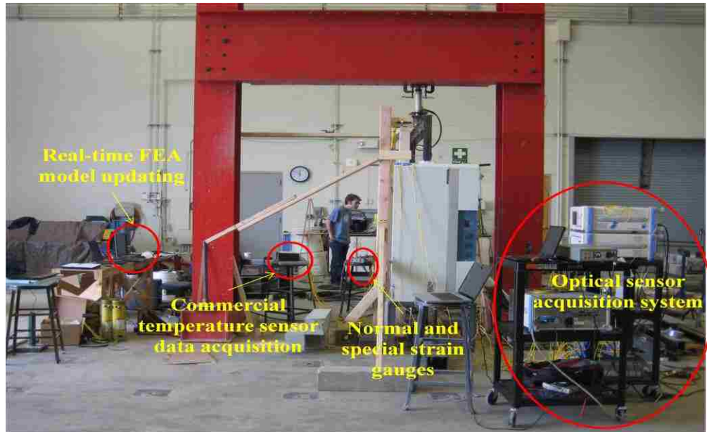
Figure 4.7 Sensing systems and network
