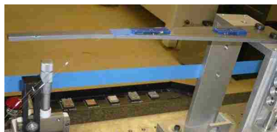
Figure 3.14 Testing of cantilevered beam
